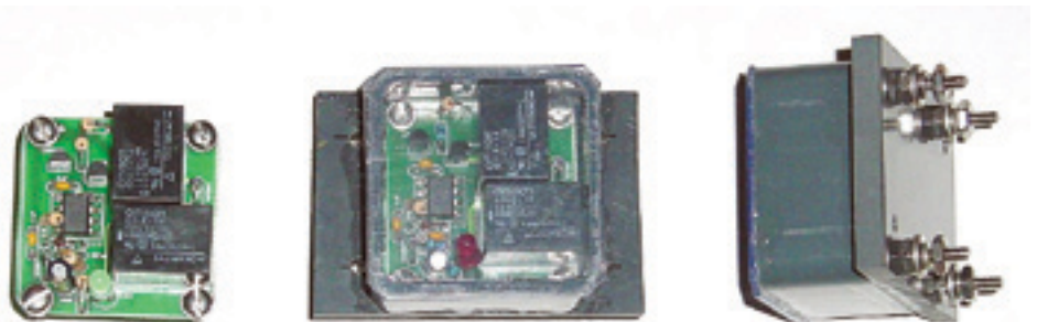
Figure 4 — Relay module. Shown is a completed PC board and front and side views of completed relay modules. The antenna wires will be connected to the studs on the back of the relay modules.
